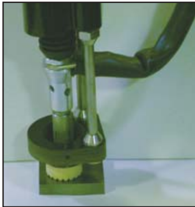
B. Locate the stud, pull the trigger, and weld is automatic
