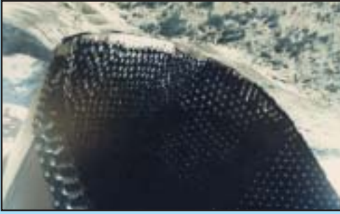
A bucket on a Bucket Wheel Reclaimer
