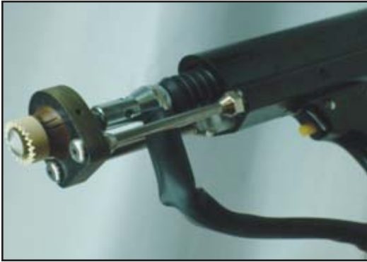
A. Operator Loads Stud & Ferrule into the hand gun
